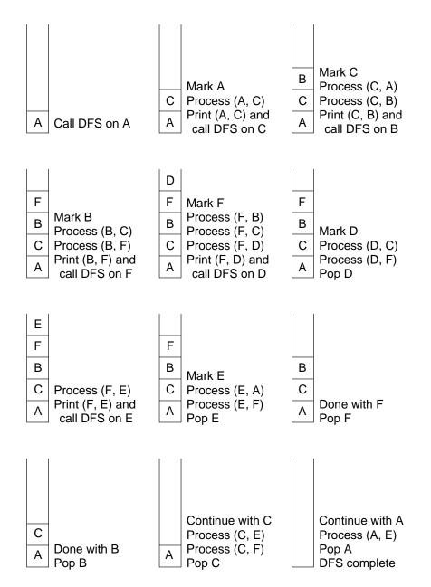
**Figure 11.9** A detailed illustration of the DFS process for the graph of Figure 11.8(a) starting at Vertex *A*. The steps leading to each change in the recursion stack are described.
