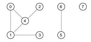
**Figure 11.2** An undirected graph with three connected components. Vertices 0, 1, 2, 3, and 4 form one connected component. Vertices 5 and 6 form a second connected component. Vertex 7 by itself forms a third connected component.
