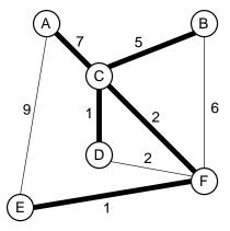
**Figure 11.20** A graph and its MST. All edges appear in the original graph. Those edges drawn with heavy lines indicate the subset making up the MST. Note that edge (C, F) could be replaced with edge (D, F) to form a different MST with equal cost.
