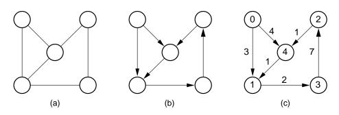
**Figure 11.1** Examples of graphs and terminology. (a) A graph. (b) A directed graph (digraph). (c) A labeled (directed) graph with weights associated with the edges. In this example, there is a simple path from Vertex 0 to Vertex 3 containing Vertices 0, 1, and 3. Vertices 0, 1, 3, 2, 4, and 1 also form a path, but not a simple path because Vertex 1 appears twice. Vertices 1, 3, 2, 4, and 1 form a simple cycle.
